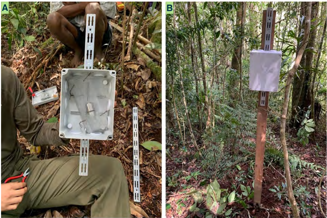
Figure 1. The weather stations were placed in rectangular plastic boxes with an open bottom and sides to protect the devices from direct solar radiation and to allow adequate ventilation. A) Protection grilles were glued in the bottom and sides of the box to prevent insects from entering. B) We attached and tied the plastic box to a horizontal wooden pole at a height of 1 m above the ground. (Photo by Lovanomenjanahary Marline.)
